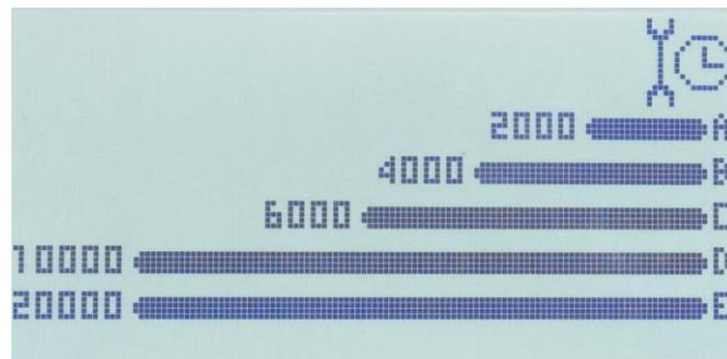
This screen shows remaining time to services A,B, C, D and E in **hours**. Service timers operate on a decremental basis. Service bars are emptied with relation to timer values.
