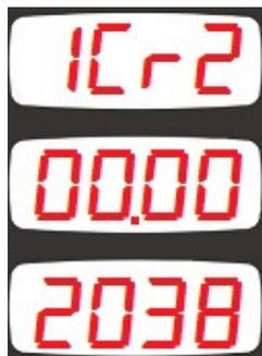
In the first current input zero mode, the first display will show "1CRZ". The second screen will display the measured instantaneous current from the input. The third display will display the offset value causing display 00.00 at no current.
