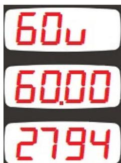
In 60V input calibration mode, the first display will show “60V”. The second screen will display the measured instantaneous voltage from the input. The third display will display the calibration coefficient (high 4 digits only)
