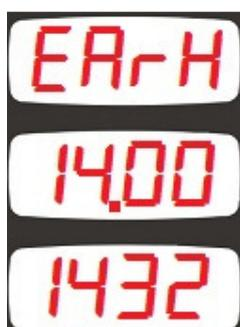
In earth voltage calibration mode, the first display will show “EarH”. The second display shows the instantaneous voltage measured at the EARTH input. The third display shows the calibration coefficient.
