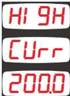
This parameter adjusts the overcurrent limit.
