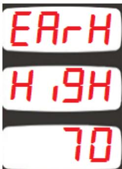
This parameter adjusts the upper limit of the ratio of the earth voltage to supply voltage.
