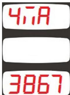
In 4mA calibration mode, the first display will show “4mA”. The second display is blank. The third display will show the calibration coefficient necessary to send 4mA from the analog output.
