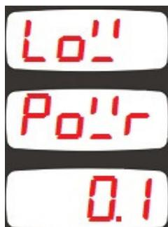
This parameter adjusts the lower limit of the low power alarm. Positive and negative powers are monitored for their absolute value and the alarm occurs for any direction of the power flow.
