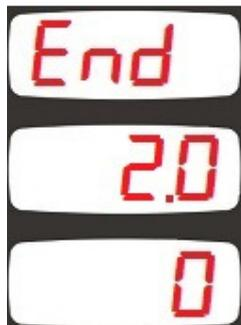
The firmware version is displayed in the second line of the “End , End” screen.
