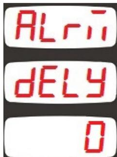
This parameter determines the delay between an alarm condition occurs and the alarm given.
