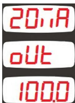
This parameter defines the value corresponding to 20mA current output. (high limit)
