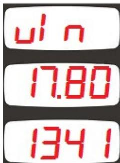
Vin voltage is generated internally and used to check that the internal power supply is operating.
