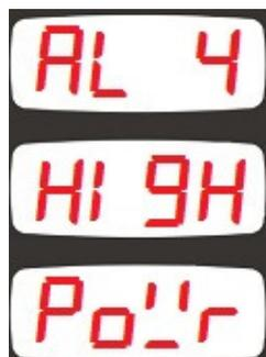
Alarm 4 : Excess Power (kW) Alarm
