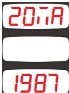
In 20mA calibration mode, the first display will show “20mA”. The second display is blank. The third display will show the calibration coefficient necessary to send 20mA from the analog output.
