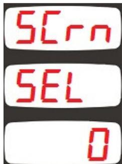
This parameter selects the screen menu where the unit returns when no pushbutton is pressed during 5 minutes.
