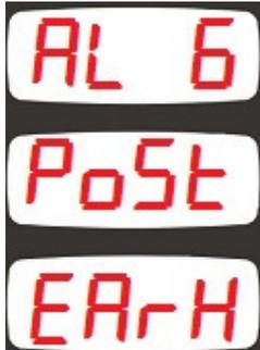
Alarm 6 : Positive (+) earth leakage alarm
