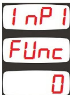
This parameter selects the function performed when the digital input\_1 signal is active.
