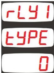
This parameter determines the RELAY\_1 contact type.
