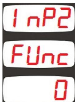
This parameter selects the function performed when the digital input\_2 signal is active.
