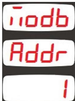
This parameter determines the Modbus node address of the unit. Every unit in the same Modbus loop must have a different node address.
