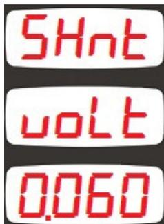
This parameter adjusts the rated voltage of the current shunt in volts.
