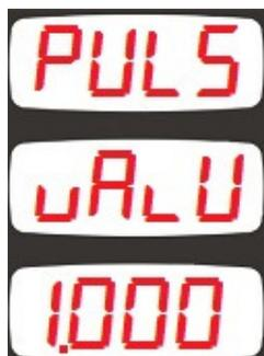
This parameter defines the counter increment step to provide 1 pulse.
