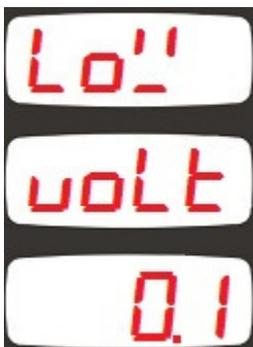
This parameter adjusts the lower limit of the low voltage alarm.
