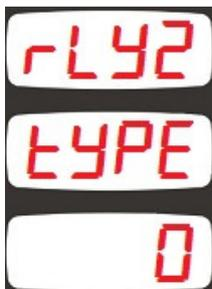
This parameter determines the RELAY\_2 contact type.
