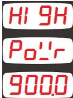
This parameter adjusts the upper limit of the high power alarm. Positive and negative powers are monitored for their absolute value and the alarm occurs for any direction of the power flow.
