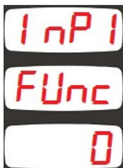
This parameter selects when the input function is activated for the digital input\_1.
