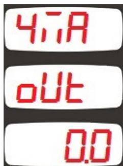
This parameter defines the value corresponding to 4mA current output. (low limit)
