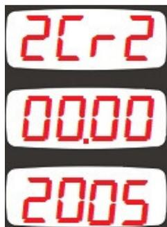
In the second current input zero mode, the first display will show "2CRZ". The second screen will display the measured instantaneous current from the input. The third display will display the offset value causing display 00.00 at no current.
