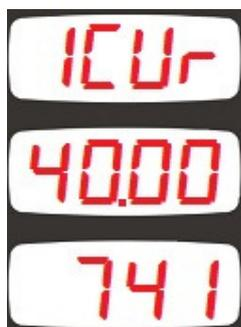
In the first current input sensitivity calibration mode, the first display will show "1CUR". The second screen will display the measured instantaneous current from the input. The third display will display the calibration coefficient (high 4 digits only)
