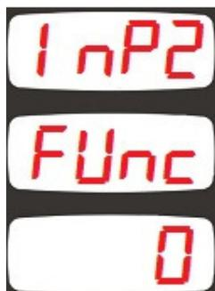
This parameter selects when the input function is activated for the digital input\_2.
