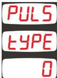
This parameter determines the counter providing pulses.
