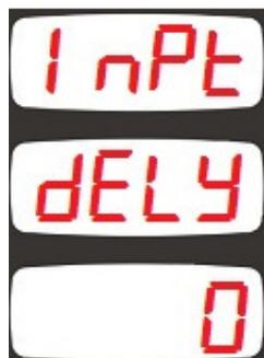
This parameter determines the wait delay between the digital input signal and the activation of input function.
