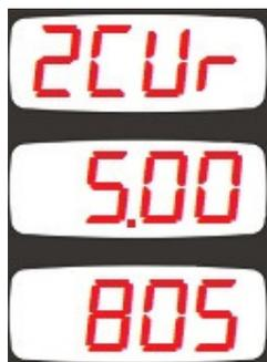
In the second current input sensitivity calibration mode, the first display will show "2CUR". The second screen will display the measured instantaneous current from the input. The third display will display the calibration coefficient (high 4 digits only)
