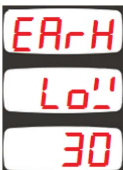
This parameter adjusts the lower limit of the ratio of the earth voltage to supply voltage.
