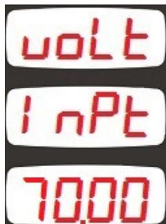
This parameter selects the voltage threshold where the voltage measurement switches from the sensitive range normal range.
