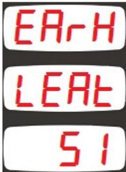
The measured earth leakage is displayed with 1% precision from both Modbus and the screen.
