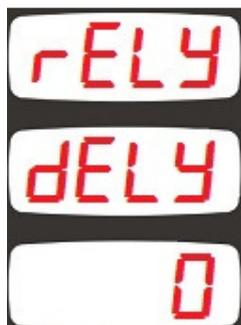
This is the wait delay between the conditions that will activate the relay occur and the relay is activated.
