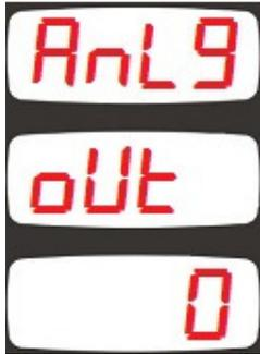
This parameter determines the analog value to be output from the 4-20mA analog output.
