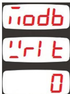
If this parameter is set to a value different from 0, then the unit will require this parameter as a password prior to Modbus writes or Modbus commands.
