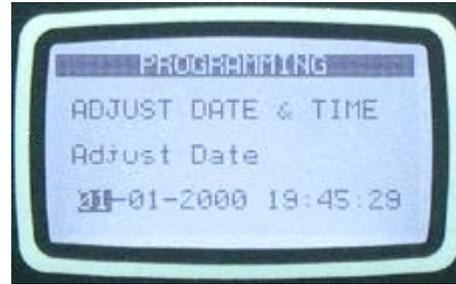
These parameters allow adjusting the battery backup real time clock of the module. Once set, the clock will continue to run even if DC power is removed from the unit.
