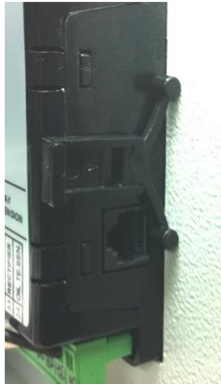
Installation of self retaining type bracket
