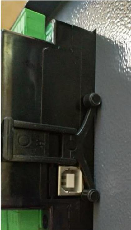
Self-retaining type bracket mounting
